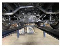
Install the Over Axle Assy. **#C** into the muffler at least 1-1/2" to 2". **#C** needs to be installed from the back of the car where the Spare Tire Sits. Use clamp **#H** to secure pipe to the muffler. Do not tighten. Insert hangers into rubber grommet.
